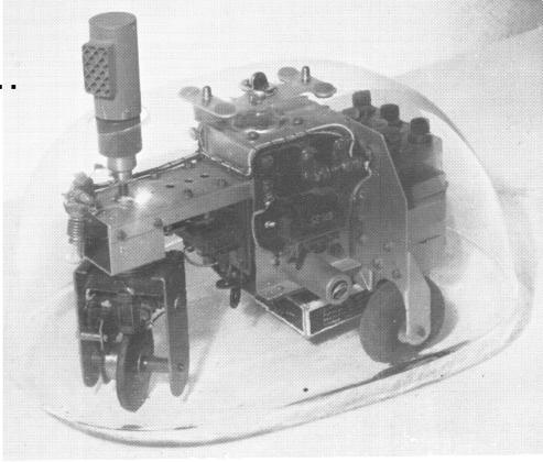
Electro-mechanical robot, Light-sensitive with Internal and External stability (ELSIE)
