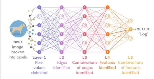
When data is fed into a network, each artificial neuron that fires (labeled "1") transmits signals to certain neurons in the next layer, which are likely to fire if multiple signals are received. The process filters out noise and retains only the most relevant features.
